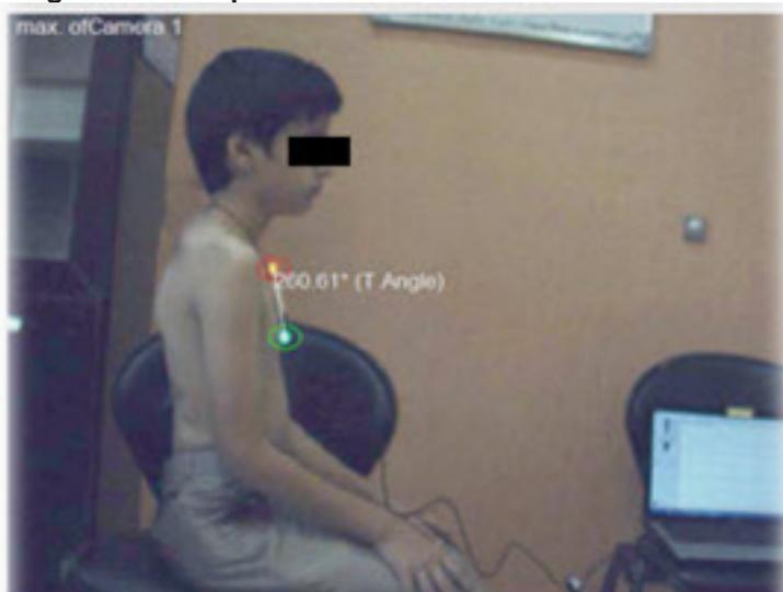
These markers can be identified by the camera and the software and the angle they make to the ground will be identified. Then the device was set on the body of the volunteer, and he sat on a table. First the correct flexion and extension movement was practiced by the volunteer and then he was asked to start doing the movements as required. Then the results and the graphs were compared. To ensure, and increasing the error rate, the measurements were repeated three
