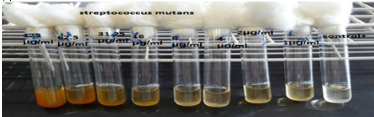
Figure 2: The adhered (sticking) cells in test tubes wall in various concentrations of curcumin. (a) Streptococcus mutans : Curcumin at a concentration of 125 µg/ml and above caused adhesion inhibition on the surfaces of the test tube (b) Lactobacillus acidophilus : Curcumin at a concentration of 31.25 µg/ml and more caused adhesion inhibition tested on the test tube surfaces.
